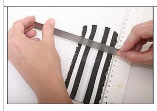
Cut the final sheet into 4-5 sections, every piece should be around 3 cm width.
